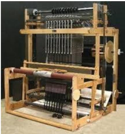
Joseph-Marie Jacquard was born in a family of weavers and invented the Jacquard Loom in 1801. The loom was invented to reduce the time spent by weavers on the job. The idea behind the Jacquard-loom was a system of punch cards and hooks. It uses a chain of punch to instruct the loom to make different fabric. For e.g. a loom can have hundreds of cards with holes corresponding to hooks that can be raised or lower to design the fabric. The Jacquard loom is
